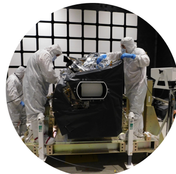
Images (Top): First published GEMS images Credit: NIER; (Bottom): GEMS Electromagnetic Interference/ Electromagnetic Compatibility (EMI/EMC) testing.
